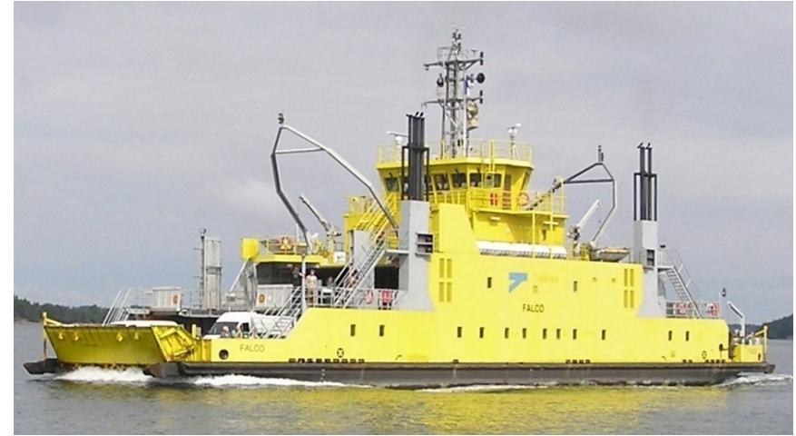
▪ Figure 3. The first autonomous ferry boat “Falco”, Finferries & Rolls-Royce, 220 cars, 3 decks, 2018 (Source: Baltic Transport Journal)
