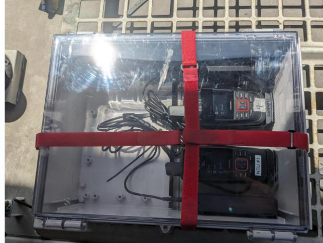
Encased GPS set on the roof of the driver's cabin
