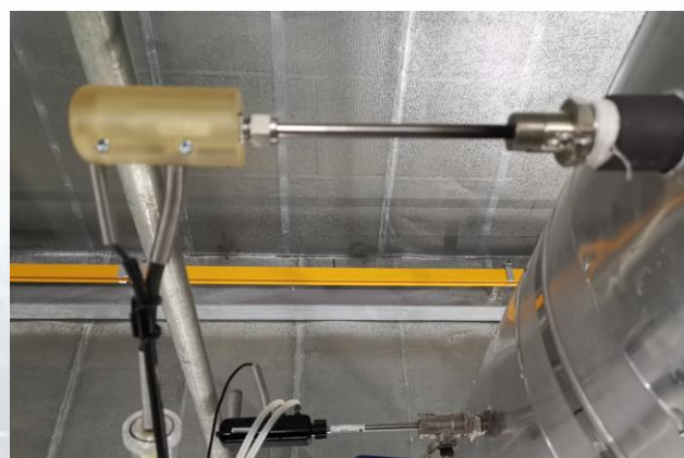
Gas analyzer's probe attached to the adapted exhaust pipe
