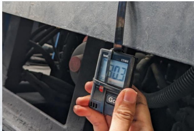
RH & Temps sensor attached on the exterior of the frame
