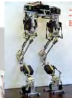
Singapore's tallest smart robot. The humanoid robot, named NASHI (NTU Advanced Smart Humanoid), learns from experience and is able to see, respond to instructions and walk up stairs.
