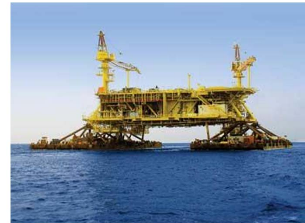
Floatover Installation for Kikeh Spar (Courtesy: Technip)
