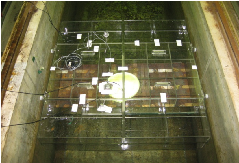
The floating breakwater equipped with oscillating water column devices
