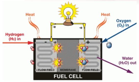
An electro-chemical device that converts hydrogen and oxygen into heat and power
